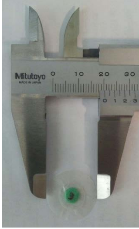
Fig. 3: Target for the ICON and LVR-15 activation prepared by evaporating \text{Mn/CoCl}_2 solution to dryness on quartz wool filter and sealing by scotch tape.
