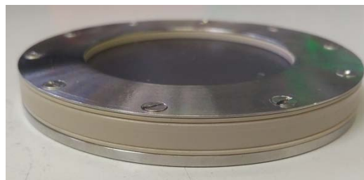
Fig. 1: Cuvette for activation of liquid targets with ultra-cold neutrons (outside diameter = 100 mm, total thickness = 13 mm).
