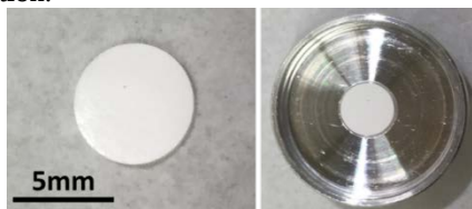
Fig. 2: Representative picture of a 6 mm target pellet made of 30 mg CaO as prepared (left) and after encapsulation in the aluminum target capsule (right).
