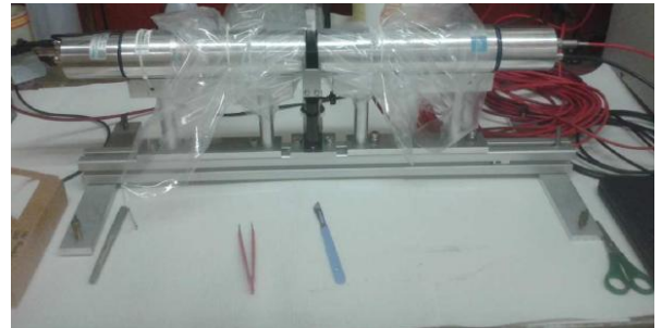
Fig. 2: Two LaBr 3 detectors were used to measure the ^{11}\text{Be} activity following the neutron irradiation of ^{10}\text{Be} .
