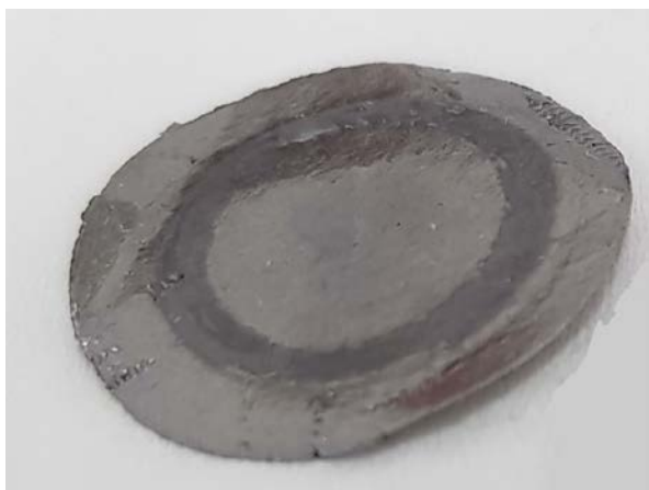
Fig. 3: Picture of Be (dark ring) electrodeposited on graphite after applying a potential of -1.8 \text{ V} for 12 hours.
