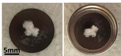
Fig. 1: Pelletized target for ^{44}\text{Sc} production as prepared with graphite powder (left) and after encapsulation in the aluminum target capsule (right).
