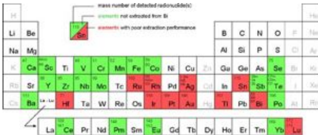
Fig. 1: Chart of detected elements indicating their extraction performance. Elements given in grey were evaporated by the 1000°C treatment.
