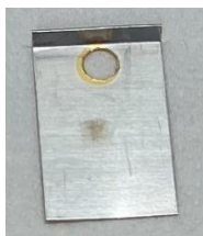
Figure 2: Al-coated gold foil implanted with Er-169. The beam spot size and shape of the Er-169 implanted area (dark grey) are visible on the Al layer close to the center of the image.
