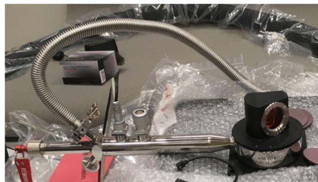
Fig. 3.8: A photograph of the cryostat system assembled and awaiting mounting for commissioning phase at the microXAS beamline.
