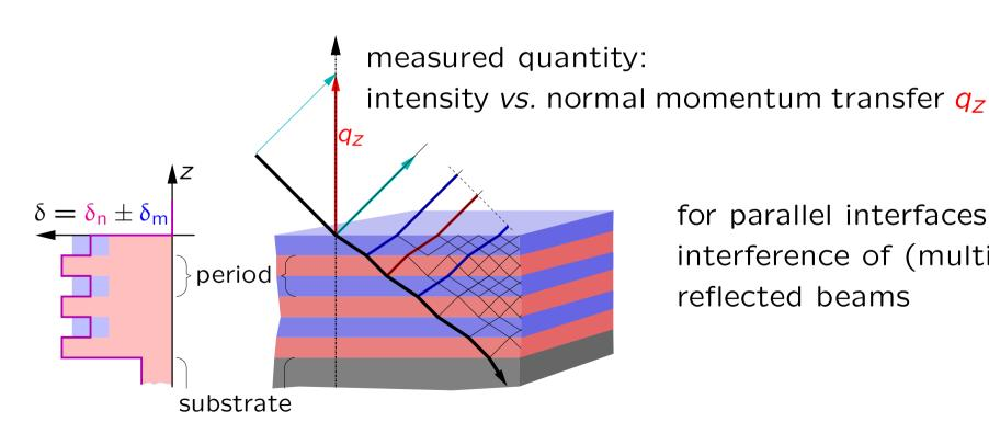
for parallel interfaces: interference of (multiply) reflected beams
