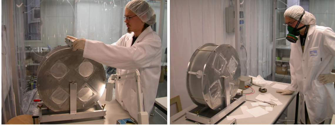
Figure 5.28: The coating device being adjusted for good 'horizontal' (left). The Rexolite ring is being rotated with some DPS solution inside until the solvent evaporates (right).
